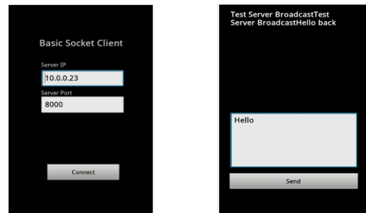
Figure 23 Android TCP Testing Interface.
