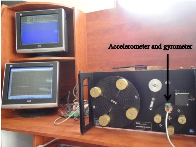
Figure 13. The sensors calibration experiments.
