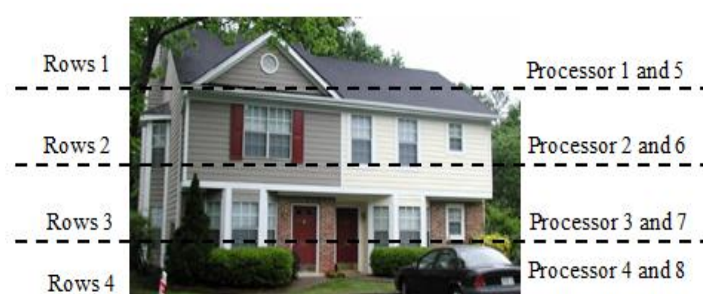
Figure 3: Example of decomposition for the image where the number of worker processors equals 8
