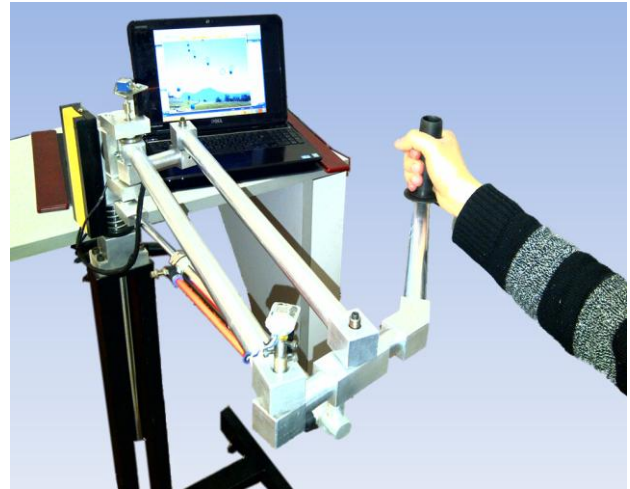
Figure 1. The whole system consisting of the mechanical arm which is driven by the patient hand and the computer where the games are displayed.
